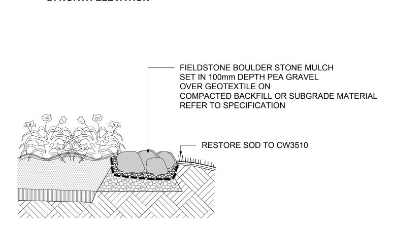
5 SECTION THROUGH STONE MULCH L1.1 | SCALE: 1:25
